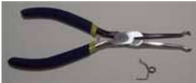
Long Nose damaged jaw
