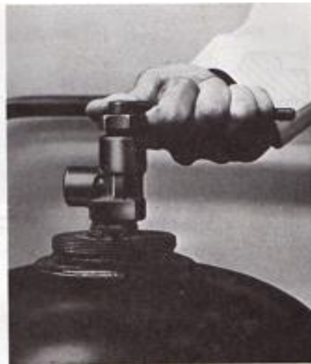
Cracking oxygen and fuel cylinder valves
