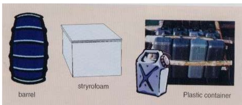
Figure 6. Commonly used materials for floaters.
