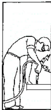
IN SOME CASES TOOLS CAN BE CHANGED TO KEEP THE ARMS LOW AND ELBOWS IN BAD DESIGN
