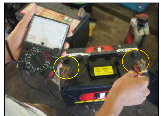
Connection of tester when testing voltage
