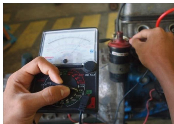
Ignition coil on test
