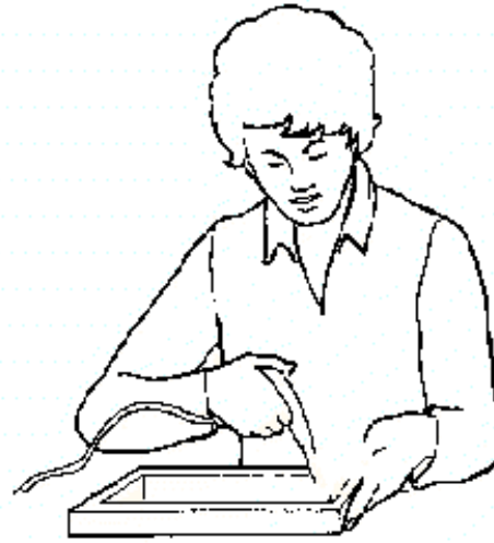
SOLDERING IRON WITH BENT HANDLE ALLOWS ELBOW TO BE LOWERED AND WRIST STRAIGHTENED GOOD DESIGN
