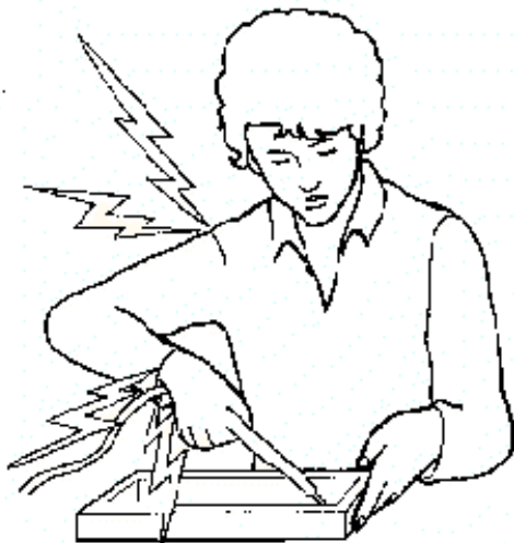
IN SOME CASES TOOLS CAN BE CHANGED TO KEEP THE ARMS LOW AND ELBOWS IN BAD DESIGN
